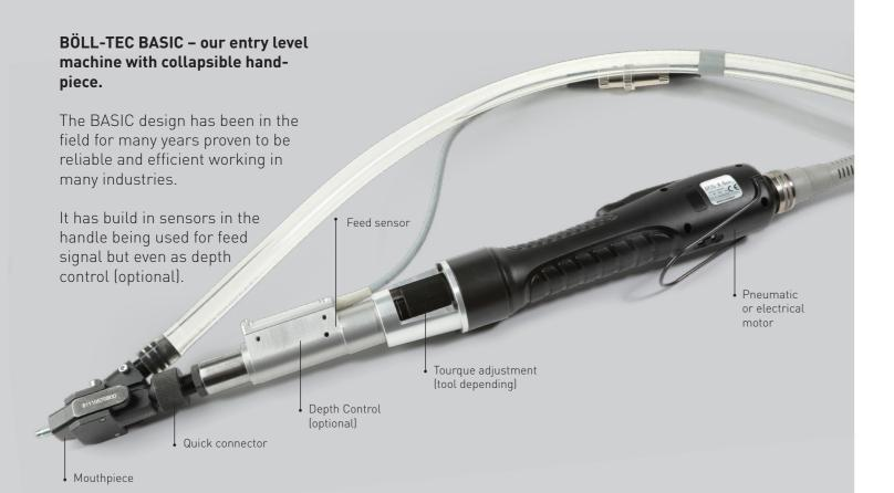
By compressing the handpiece the motor is started (by push start) and the Jaws (mouthpiece) are engaged to the surface while the screw is inserted. Due to this system it is not to be used in operation with delicate surface. It is ideal for general industry like wood, sheetmetal and similar.
